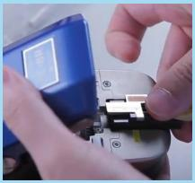
Remove and slit the cord sheath using the Lynx strip & slit tool.
