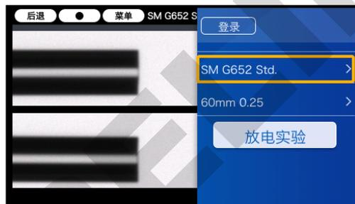
2) 用(▼▲)键移动光标
